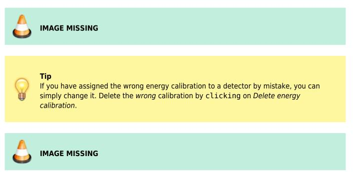
Open the valid calibration measurement of the detector and reevaluate the measurement (even of you have not changed any analysis parameters! It is important that the *Save* button is activated again). If you subsequently click on *Save*, you will be asked again whether you would like to use this calibration for the detector. The same applies to efficiency calibrations and linking of parameter sets.
